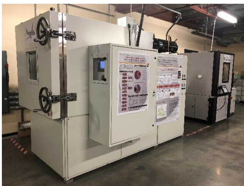
Figure 8 Specialized equipment to simulate land and air transportation
