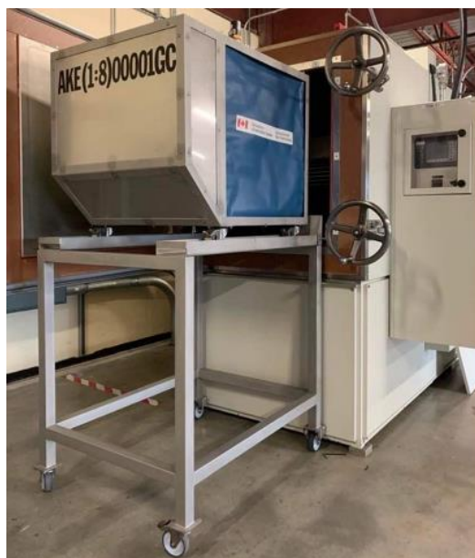
Figure 25 AKE with a scale size factor of 1:8 being loaded inside an altitude test chamber for the simulation of an air shipment (credit: AAFC).
