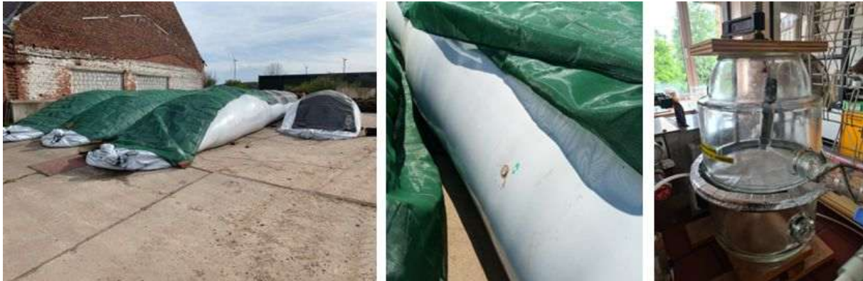
Figure 22 Silo bags on a farm (left). Oxygen measurements were taken with a syringe through a septum (center). The oxygen permeability of the silo foil was tested in the lab (right) (Photos: C. Müller-Blenkle, JKI)
