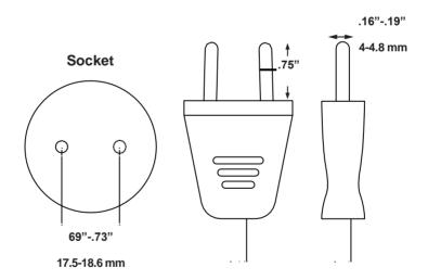
**Dimensions Guide Type D Plug & Socket**
